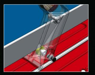
CARRIAGE Carriage provided with adjustable ball-bearing for getting a perfect sliding and top precision.
