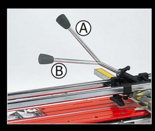
To optimize the cutting and breaking phase, turn and lock the handling lever into the "A" or "B" position, according to the tiles' thickness as following:
