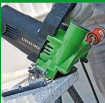
Cutting large-format slabs, mitre cuts up to 45°
