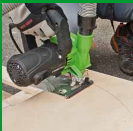
Curved cuts with diamond concave disc
