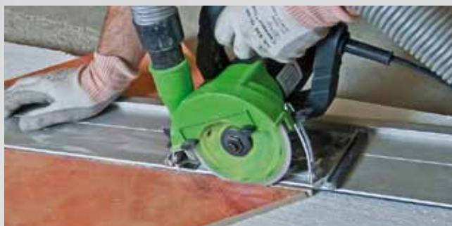
Machine on guide rail – for precise cuts, unlimited extensions
