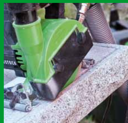
milling of joints with diamond milling disc – depth limiting and immersion function
