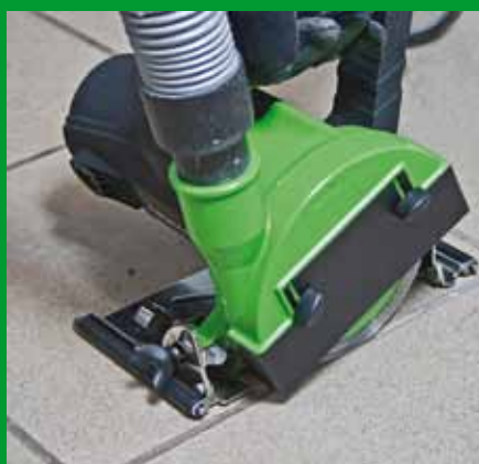
Joint milling – dry cutting with depth limiting and immersion function
