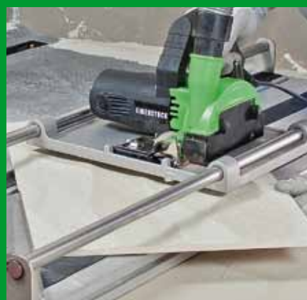
Diagonal cut with cutting table
